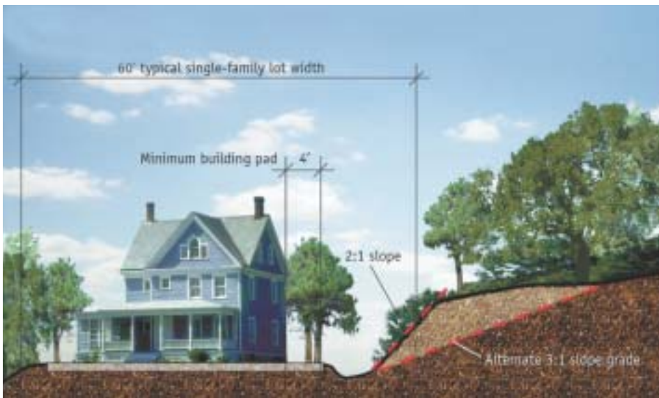
A two-to-one slope will save more existing vegetation than the more conventional three-to-one slope, which disturbs more of the natural topography and thus removes more trees.
